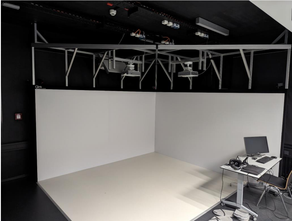
Figure 4: VR Corner Cave at the faculty of maritime sciences of the University of Applied Sciences Emden/Leer
